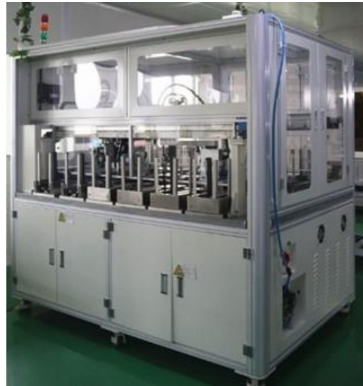
▲ Automated sorting equipment
